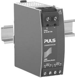
The YR80.241 is equipped with two input channels (40A each), which are individually decoupled by utilizing mosfet technology. The output current can go as high as 80A.
