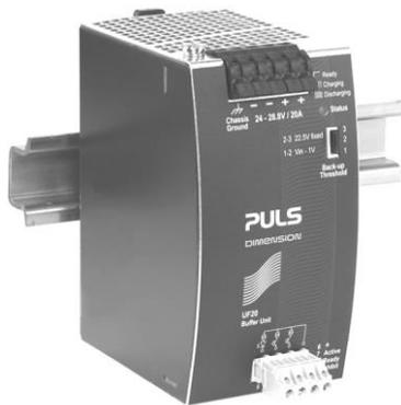
This buffer unit is a supplementary device for DC 24V power supplies. It delivers power to bridge typical mains failures or extends the hold-up time after turn-off of the AC power. In times when the power supply provides sufficient voltages, the buffer unit stores energy in integrated electrolytic capacitors. In case of mains voltage fault, this energy is released again in a regulated process.
