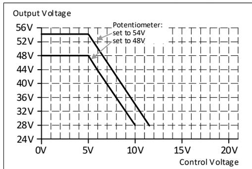
Fig. 10-2 Applying the control voltage
