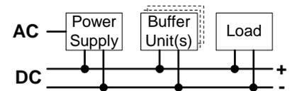
The buffer unit does not require any control wiring. It can be added in parallel to the load circuit at any given point. Buffer units can be added in parallel to increase the output ampacity or the hold-up time.
