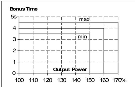
Fig. 6-4 Dynamic overcurrent capability, typ.
