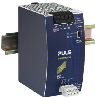
This buffer unit is a supplementary device for DC 48V power supplies. It delivers power to bridge typical mains failures or extends the hold-up time after turn-off of the AC power. In times when the power supply provides sufficient voltages, the buffer unit stores energy in integrated electrolytic capacitors. In case of mains voltage fault, this energy is released again in a regulated process.
