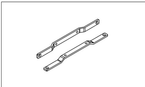
Fig. 23-4 Wall mounting with DIN rail brackets\*)
