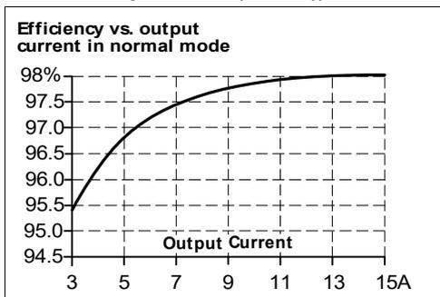
Fig. 8-2 Losses at 24V, typ.
