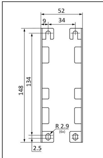
Fig. 23-10 Wall/panel mounting, side view
