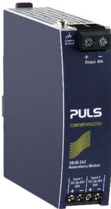
The YR40.242 is the preferred redundancy module for PIC480.241C power supplies. It is equipped with two input channels (20A each), which are individually decoupled by utilizing MOSFET technology. The output current can go as high as 40A.
