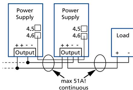
Fig. 18-1: Daisy chaining of outputs
