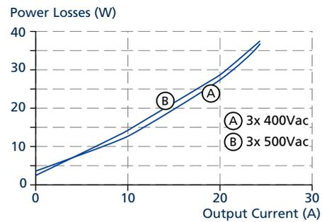
Fig. 14-2: Losses vs. output current at 48 V, typ.
