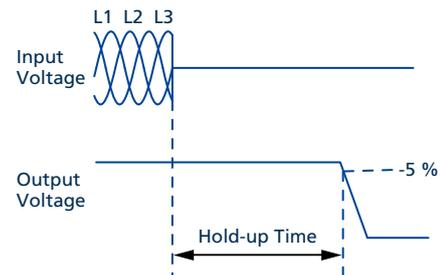
Fig. 8-2: Shut-down behaviour
