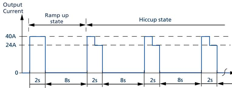
Fig. 7-3: Short-circuit on output, Hiccup<sup>PLUS</sup> mode, typ.
