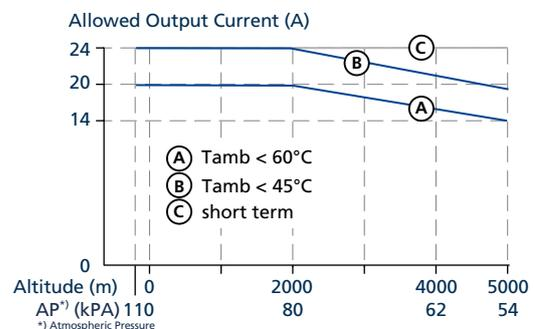
Fig. 22-2: Output current vs. altitude
