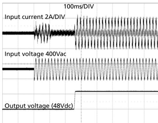
Fig. 6-1: Typical turn-on behaviour at nominal load and +25 °C ambient<sup>1</sup>
