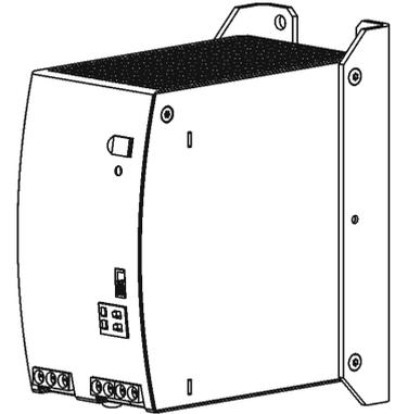
Due to the small size of the unit, it is required that the black-DIN rail slide on the back of the unit must be removed. Instructions how to do this can be found in the manual of the ZM2.WALL.
