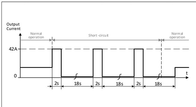
**Fig. 6-4 Dynamic overcurrent capability, typ.**
