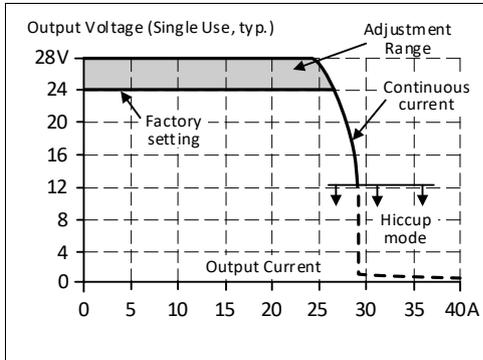
**Fig. 6-2 Output voltage in "parallel use" mode, typ.**
