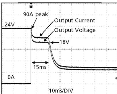
High Overload Current (typ. >90A for 15ms) enables easy fuse tripping
