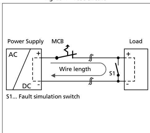
Maximal wire length<sup>\*)</sup> for a fast (magnetic) tripping:
