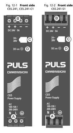
**Input Terminals** CS5.241, CS5.241-C1 with screw terminals CS5.241-S1 with spring-clamp terminals N, L Line input ٢ PE (Protective Earth) input **<u>B</u>** Output Terminals (screw terminals, two pins per pole) Positive output + Negative (return) output **<u>C</u>** Output voltage potentiometer Open the flap to adjust the output voltage. Factory set: 24.1V D DC-OK LED (green)
