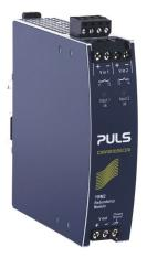
The YRM2.DIODE is a dual redundancy module, which can be used to build redundant systems. It is equipped with two input channels, which are individually decoupled by utilizing diodes.
