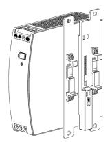
Side mounting with DIN rail brackets
