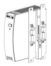
Side mounting with DIN rail brackets
