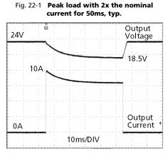
10A Peak load (resistive) for 50ms Output voltage dips from 24V to 18.5V.
