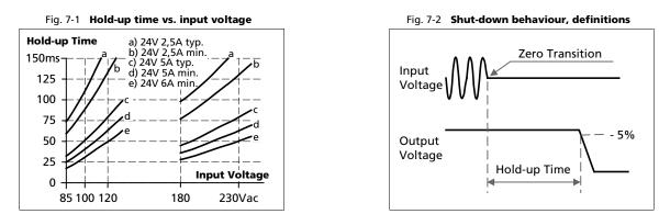
At no load, the hold-up time can be up to several seconds. The green DC-OK LED is on during this time. Note:
