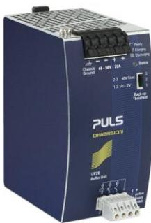
This buffer unit is a supplementary device for DC 48V power supplies. It delivers power to bridge typical mains failures or extends the hold-up time after turn-off of the AC power. In times when the power supply provides sufficient voltages, the buffer unit stores energy in integrated electrolytic capacitors. In case of mains voltage fault, this energy is released again in a regulated process.
