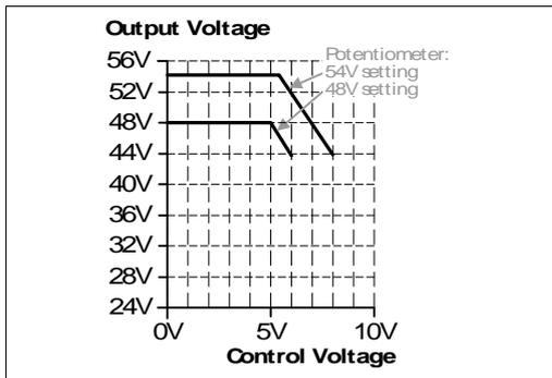
Fig. 10-2 Applying the control voltage
