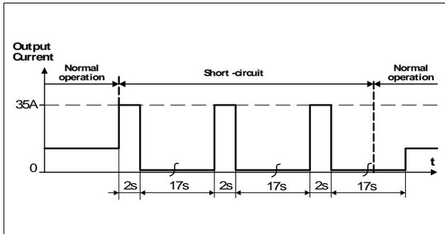
Fig. 6-4 Dynamic overcurrent capability, typ.
