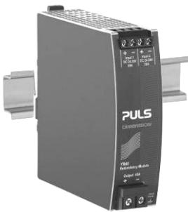
The YR40.241 redundancy module is equipped with two input channels (20A each), which are individually decoupled by utilizing MOSFET technology. The output current can go as high as 40A.
