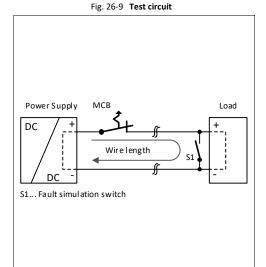
Maximal wire length\*) for a fast (magnetic) tripping:
