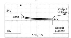
200A Peak load (resistive) for 5ms Output voltage dips from 24V to 17V.
