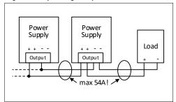
Fig. 15-2 Using distribution terminals
