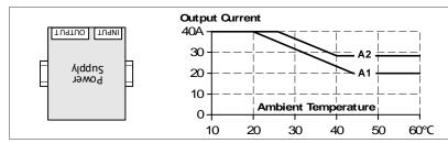
Fig. 26-12 Mounting Orientation C (Table-top mounting)
