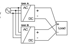
Keep an installation clearance of 15mm (left / right) between two power supplies and avoid installing the power supplies on top of each other. Do not use power supplies in parallel in mounting orientations other than the standard mounting orientation (terminals on the bottom of the unit) or in any other condition where a derating of the output current is required (e.g. altitude, above +60°C, ...).
