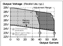
Fig. 6-4 Dynamic overcurrent capability, typ.
