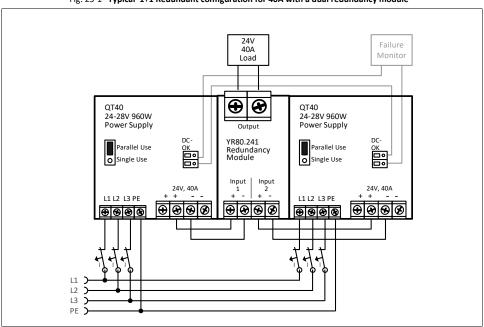
Fig. 25-1 Typical 1+1 Redundant configuration for 40A with a dual redundancy module
