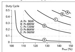
$$DutyCycle = \frac{T_{peak}}{T_{peak} + T_0}$$
