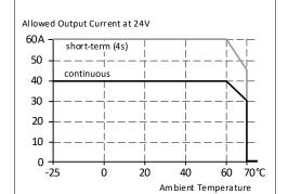
$\label{eq:Fig. 18-1} \textbf{Output current vs. ambient temp.}$
