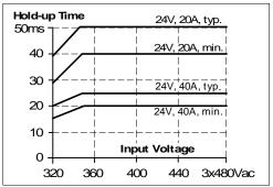
Fig. 7-2 Shut-down behaviour, definitions
