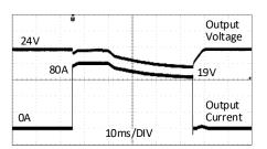
80A Peak load (resistive) for 50ms Output voltage dips from 24V to 19V.
