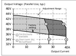
Fig. 6-4 Dynamic overcurrent capability, typ.
