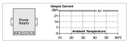
Fig. 26-11 Mounting Orientation B (Upside down)
