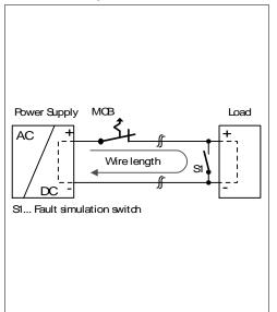
maximal wire length\*) for a fast (magnetic) tripping:
