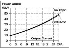
Fig. 12-4 Losses vs. input voltage at 36V, 26.7A, typ.
