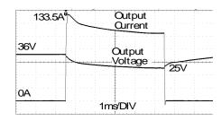
133.5A Peak load (resistive) for 5ms Output voltage dips from 36V to 25V.
