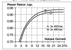
Aug. 2024 / Rev. 3.1 DS-QT40.361-EN All parameters are specified at 36V, 26.7A, 3x400Vac, 25°C ambient and after a 5 minutes run-in time unless otherwise noted.
