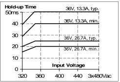
Fig. 7-2 Shut-down behaviour, definitions
