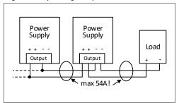
Fig. 15-2 Using distribution terminals
