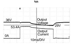
53.4A Peak load (resistive) for 50ms Output voltage dips from 36V to 29V.
