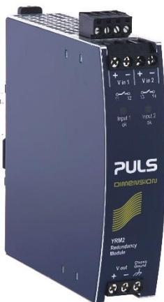
The YRM2.DIODE is a dual redundancy module, which can be used to build 1+1 and N+1 redundant systems. It is equipped with two input channels, which are individually decoupled by utilizing diodes.
