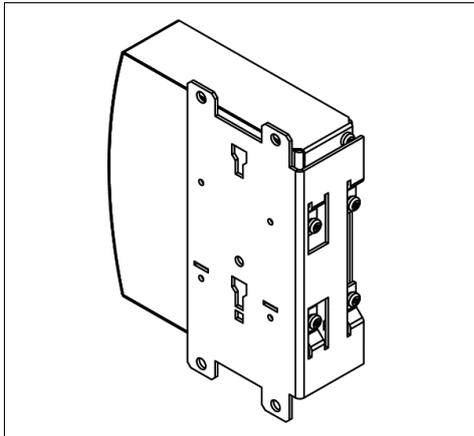
Fig. 21-6 Side mounting with DIN rail brackets\*)
