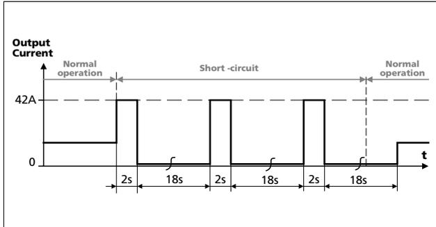
Fig. 6-4 **Dynamic overcurrent capability, typ.**
