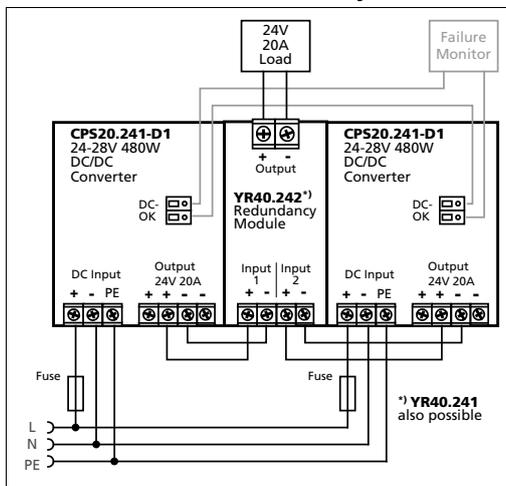
Fig. 21-2 Typical N+1 or 1+1 Redundant configuration for 20A with multiple YR40.245 redundancy modules
