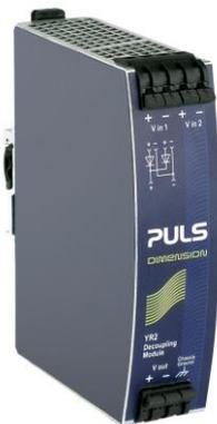
The YR2.DIODE is a dual redundancy module, which has two diodes with a common cathode included. It can be used for various purposes. The most popular application is to configure highly reliable and true redundant power supply systems. Another interesting application is the separation of sensitive loads from non-sensitive loads. This avoids the distortion of the power quality for the sensitive loads which can cause controller failures.
