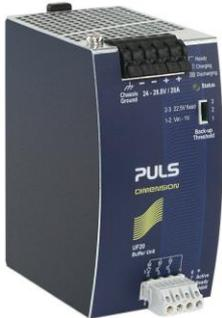
This buffer unit is a supplementary device for DC 24V power supplies. It delivers power to bridge typical mains failures or extends the hold-up time after turn-off of the AC power. In times when the power supply provides sufficient voltages, the buffer module stores energy in integrated electrolytic capacitors. In case of mains voltage fault, this energy is released again in a regulated process. One buffer module can deliver 20A which can also be used to support peak current demands.
