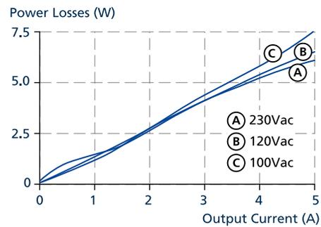
Fig. 8-2: Losses vs. output current at 12V, typ.
