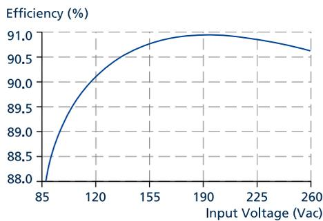
Fig. 8-3: Efficiency vs. input voltage at 12V, 5A, typ.
