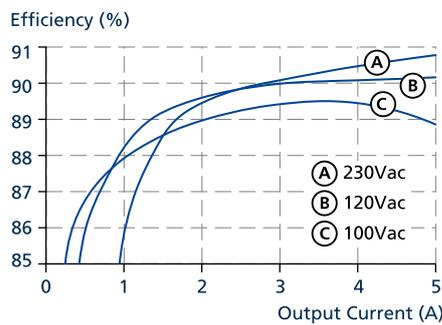
Fig. 8-1: Efficiency vs. output current at 12V, typ.
