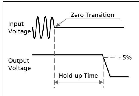
Note: At no load, the hold-up time can be up to several seconds. The green DC-OK LED is on during this time.
