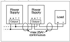
Fig. 11-2 Using distribution terminals
