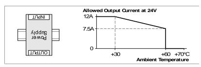
Fig. 22-12 Mounting Orientation C (Table-top mounting)
