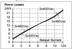
Fig. 8-4 Losses vs. input voltage at 24V, 10A, typ., 3-phase operation
