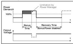
The BonusPower is available as soon as power comes on and immediately after the end of an output short circuit or output overload.
