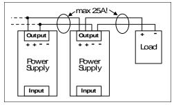
Fig. 12-3 Using distribution terminals
