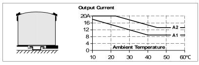
Fig. 23-9 Mounting Orientation D (Horizontal cw)
