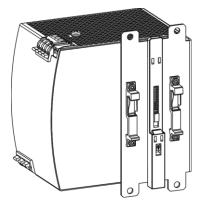
Side mounting with DIN rail brackets
