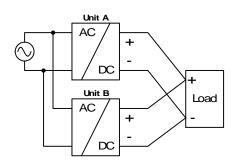
Pay attention that leakage current, EMI, inrush current, harmonics will increase when using multiple power supplies.
