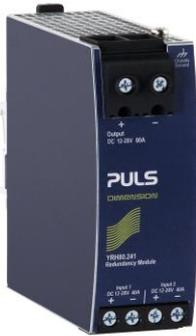
The YR80.241 is equipped with two input channels (40A each), which are individually decoupled by utilizing MOSFET technology. The output current can go as high as 80A.
