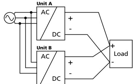
If more than three units are connected in parallel, a fuse or circuit breaker with a rating of 32A or 40A is required on each output. Alternatively, a diode or redundancy module can also be utilized.
