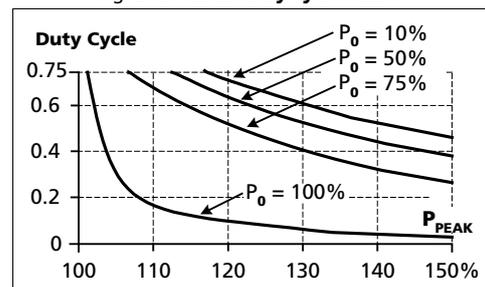
$$\text{DutyCycle} = \frac{T_{\text{peak}}}{T_{\text{peak}} + T_0}$$
