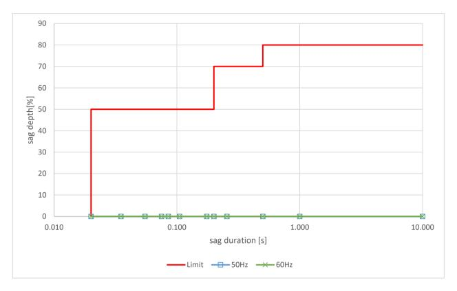
For all Sag times the voltage can be reduced to 0V without any influence on the output.
