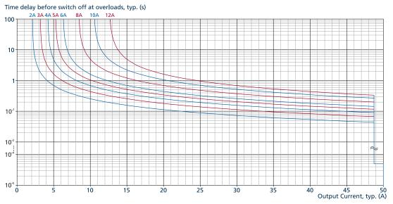
Fig. 6-3: Trip curve diagram
