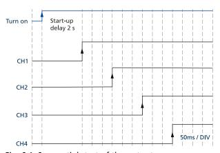
Fig. 6-1: Sequential start of the outputs
