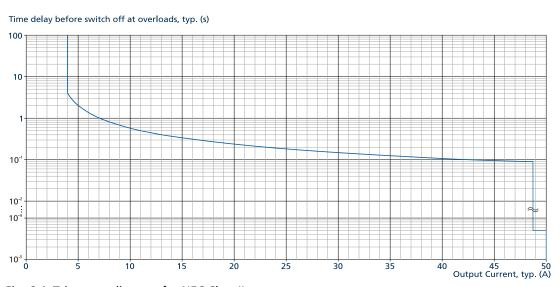
Fig. 6-4: Trip curve diagram for NEC Class II
