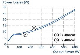
Fig. 9-2: Losses vs. output power at 24 V, typ.
