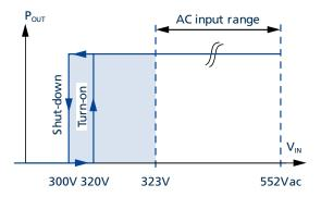
Fig. 3-1: Input voltage range
