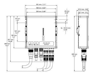
Width 181mm / 7.17" Height 183mm / 7.2" Depth 59mm / 2.32" Weight 1200g / 2.7lb Housing body material Housing cover material Installation clearances Mating connectors Aluminium alloy Hi-grade polycarbonate See chapter 2 See chapter 21.3
