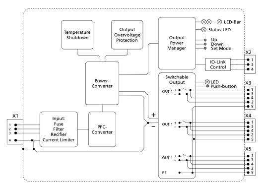
Fig. 12-1: Functional Diagram
