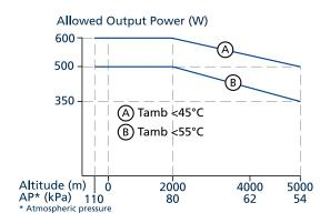
Fig. 16-2: Output power vs. altitude
