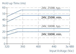
Fig. 7-1: Hold-up time vs. input voltage
