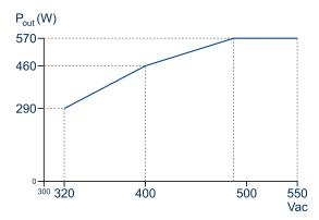
Fig. 23-1: Two phase power capability
