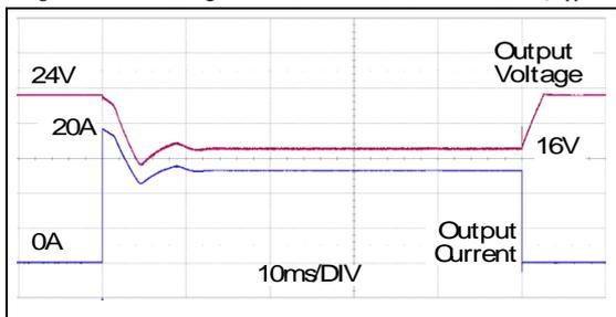
Peak load 20A (resistive load) for 50ms
