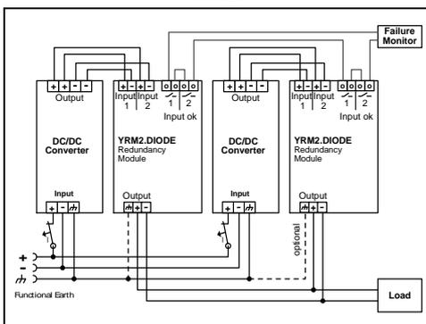
Fig. 22-5 N+1 Redundant configuration for 30A load current with multiple DC/DC converters and redundancy modules
