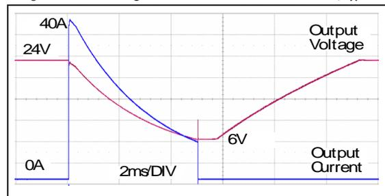
Peak load 40A (resistive load) for 5ms
