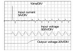
Fig. 5-2 Input inrush current, zoom into first peak 230Vac input, 24V 5A output, 25°C ambient
