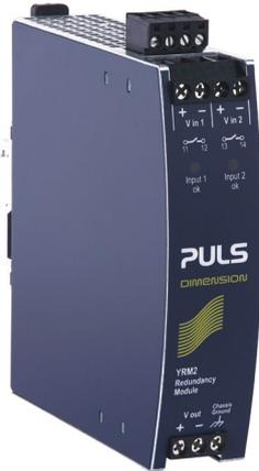
The YRM2.DIODE is a dual redundancy module, which can be used to build redundant systems. It is equipped with two input channels, which are individually decoupled by utilizing diodes.
