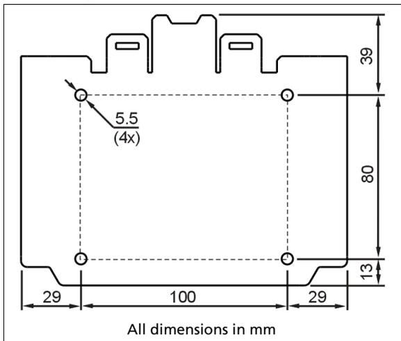
Fig. 12-3 **Hole pattern for bottom mount**
