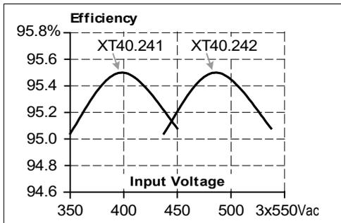
Fig. 7-4 Losses vs. input voltage, 24V, 40A
