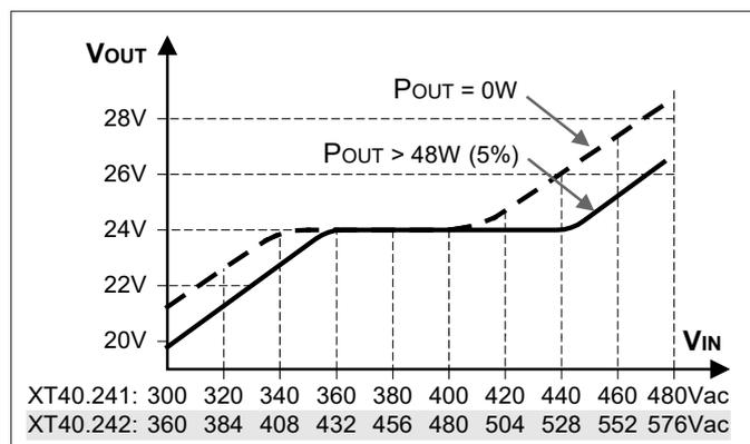
Fig. 3-2 Input voltage range
