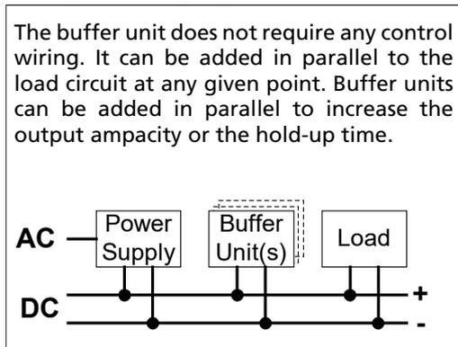
Do not use the buffer module to bridge mains interruptions which are longer than typ. 350ms. Once the mains is off for longer than typ. 350ms, the XT power supply needs an additional 1s to restart again.
