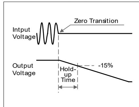
Fig. 6-2 Hold-up time vs. input voltage
