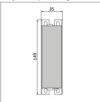
Fig. 22-5 Hole pattern for wall mounting
