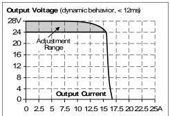
Fig. 5-3 Short-circuit on output,  $Hiccup^{PLUS}$  mode, typ.
