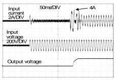
Fig. 4-2 Typical turn-on behaviour at nominal load, 230Vac input and 25°C ambient
