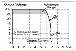
Fig. 5-2 Dynamic output current capability, typ.
