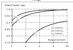
Feb. 2024 / Rev.1.1 DS-CP5.241-M1-EN All parameters are typical values specified at 230Vac, 50Hz input voltage, 24V, 5A output load, 25°C ambient and after a 5 minutes run-in time unless otherwise noted.
