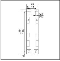
Fig. 22-6 Wall/panel mounting,
