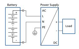
Fig. 4-1: Wiring for DC Input
