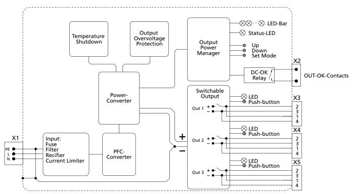
Fig. 12-1: Functional Diagram FPS300.245-049-102
