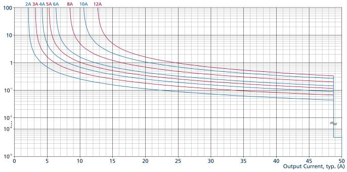
Fig. 6-2: Tripping curve diagram
