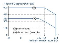
Fig. 16-1: Output power vs. ambient temp.
