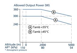
Fig. 16-2: Output power vs. altitude
