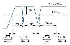
Fig. 8-1: Output-OK relay contact behavior
