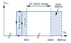
Fig. 3-1: Input voltage range
