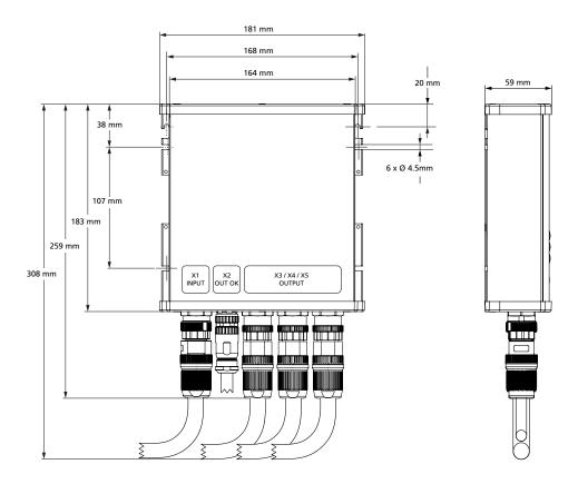
Width: 181 mm Height: 183 mm Depth: 59 mm Weight: 1200 g Housing body material: Housing cover material: Installation clearances: Aluminium alloy Hi-grade polycarbonate See chapter 2
