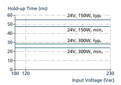
Fig. 7-1: Hold-up time vs. input voltage
