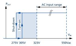
Fig. 3-1: Input voltage range
