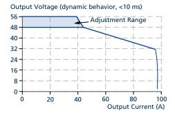
Fig. 7-2: Dynamic overcurrent capability, typ.
