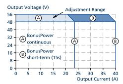
Fig. 7-1: Output voltage vs. output current, typ.
