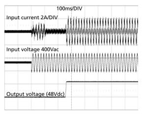
Fig. 6-1: Typical turn-on behaviour at nominal load and +25 °C ambient<sup>1</sup>
