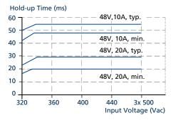
Fig. 8-1: Hold-up time vs. input voltage
