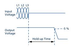
Fig. 8-2: Shut-down behaviour
