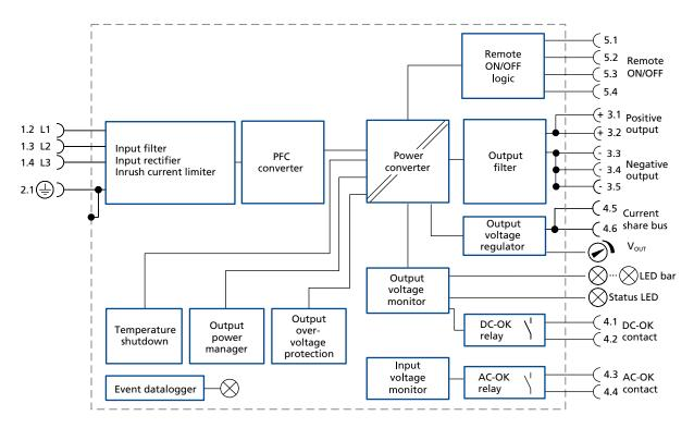
Fig. 17-1: Functional Diagram TP960.484
