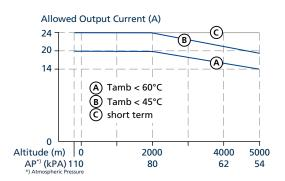
Fig. 22-2: Output current vs. altitude
