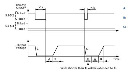
Fig. 12-1: Case 1: Pin 5.1 und Pin 5.2 linked, power supply on
