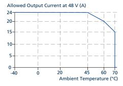
Fig. 22-1: Output current vs. ambient temp.
