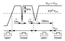
Fig. 9-1: DC OK relay contact behaviour
