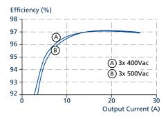
Fig. 14-1: Efficiency vs. output current at 48 V, typ.
