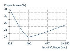
Fig. 14-4: Losses vs. input voltage at 48 V, 20 A, typ.
