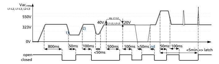
Fig. 10-1: AC OK relay contact behavior
