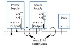
Fig. 18-1: Daisy chaining of outputs
