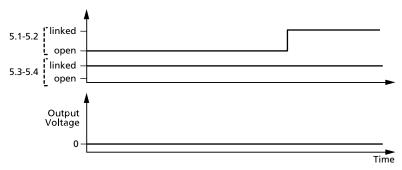
Fig. 12-3: Case 3: Pin 5.3 und Pin 5.4 linked, power supply off
