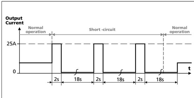
Fig. 6-4 **Dynamic overcurrent capability, typ.**
