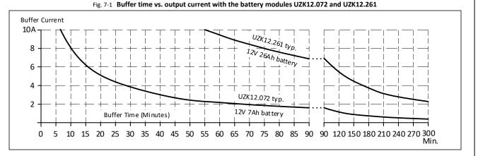
The battery capacity is usually specified in amp-hours (Ah) for a 20h discharging event. The battery discharge is non-linear (due to the battery chemistry). The higher the discharging current, the lower the appropriable battery capacity. The magnitude of the reduction depends on the discharging current as well as on the type of battery. High current battery types can have up to 50% longer buffer times compared to regular batteries when batteries will be discharged in less than 1 hour.
