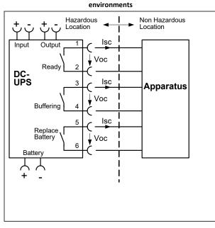
Fig. 11-1 Contact control drawing for use in Haz-Loc
