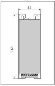
Fig. 24-7 Hole pattern for wall mounting
