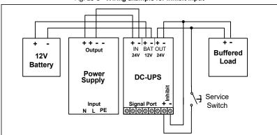
Fig. 25-3 Wiring example for inhibit input
