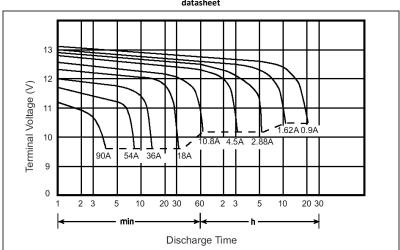
Fig. 7-2 Typical discharging curve of a typical 17Ah battery, curve taken from a manufacturer's datasheet
