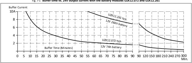
Fig. 7-1 Buffer time vs. 24V output current with the battery modules UZK12.072 and UZK12.261
