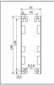
Fig. 24-8 Wall/panel mounting, side view
