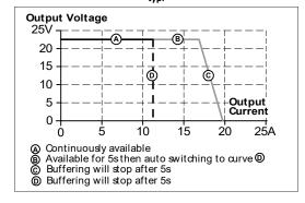
Fig. 5-5 12V Output voltage vs. output current in normal or buffer mode, typ.
