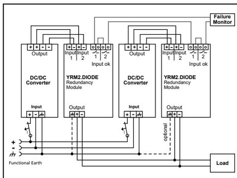
Fig. 22-5 N+1 Redundant configuration for 30A load current with multiple DC/DC converters and redundancy modules
