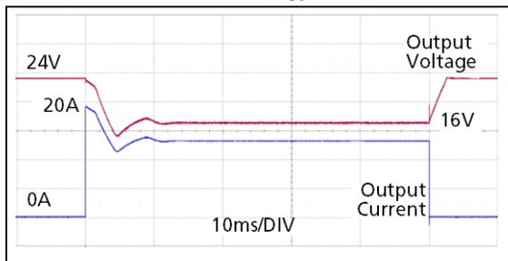
Peak load 20A (resistive load) for 50ms
