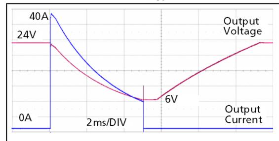
Peak load 40A (resistive load) for 5ms
