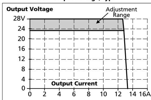
Fig. 6-2 Current limitation vs. input voltage, (23V constant voltage load), typ.
