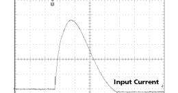
Fig. 5-2 Input inrush current, zoom into first peak
