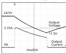
Peak load 3.15A (resistive load) for 5ms Output voltage dips from 24V to 11.5V.
