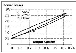
Fig. 8-4 Losses vs. input voltage at 24V, 0.63A, typ.
