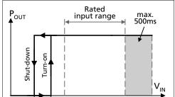
Fig. 3-1 Input voltage range
