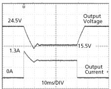
Peak load 1.3A (resistive load) for 50ms Output voltage dips from 24V to 15.5V.
