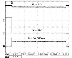
Parameters: Power supply: 5A (CS5.241) I0 = 0A I3 = Short-circuit I1, I2, I4 = 0A
