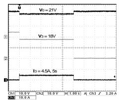
Parameters: Power supply: 5A (CS5.241) I0 = 4A (6 Ohm) I3 = 6A (4 Ohm) I1, I2, I4 = 0A
