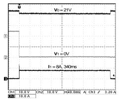
Parameters: Power supply: 5A (CS5.241) I0 = 0A I1 = Short circuit I2, I3, I4 = 0A
