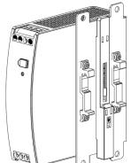
Side mounting without DIN rail brackets
