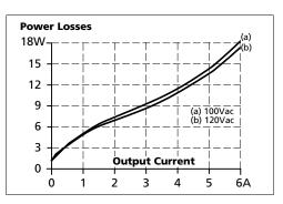
Fig. 8-4 Losses vs. input voltage at 24V, 5A,
