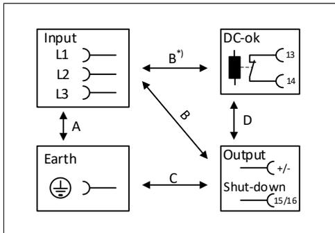
B\*) When testing input to DC-OK ensure that the max. voltage between DC-OK and the output is not exceeded (column D). We recommend connecting DC-OK pins and the output pins together when performing the test.
