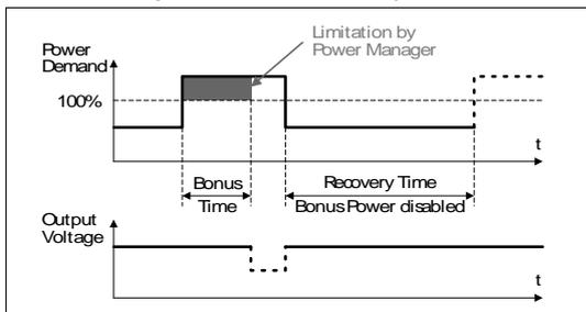
The BonusPower is available as soon as power comes on and after the end of an output short circuit or output overload.
