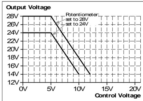
Fig. 10-2 Applying the control voltage
