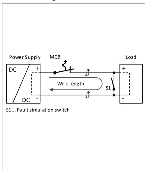
Maximal wire length<sup>\*)</sup> for a fast (magnetic) tripping:
