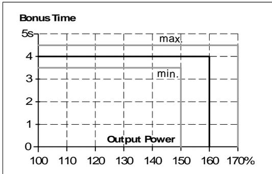
Fig. 6-4 Dynamic overcurrent capability, typ.
