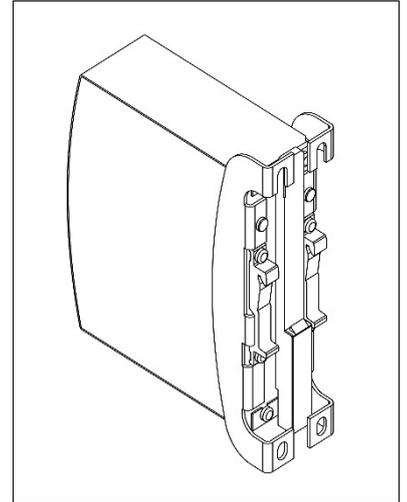
Fig. 24-4 **Wall/panel mounting, front view**
