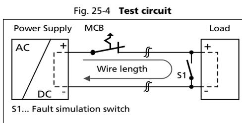
Maximal wire length<sup>\*)</sup> for a fast (magnetic) tripping:
