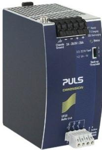
The UF20.241 buffer module is a supplementary device for DC 24 V power supplies. It delivers power to bridge typical mains failures or extends the hold-up time after the AC power is turned off.
