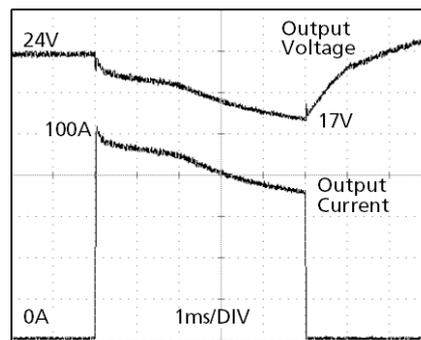
Fig. 25-3 **60 A<sub>peak</sub> current for 12 ms, typ.**
