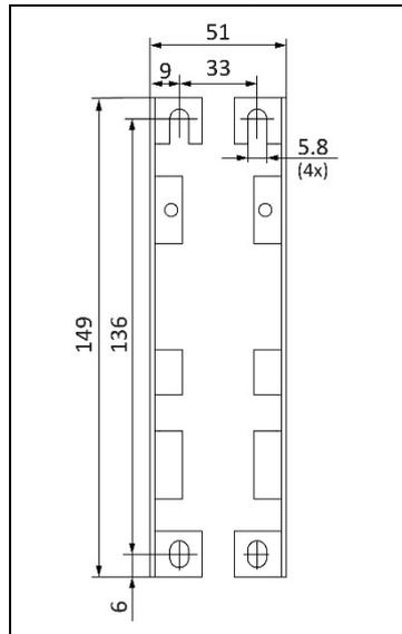
Fig. 24-6 **Wall/panel mounting, side view**
