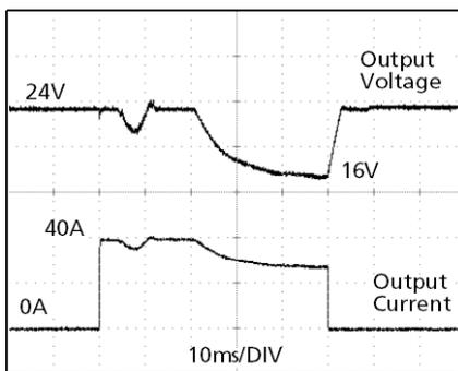
Fig. 25-2 **100 A<sub>peak</sub> current for 5 ms, typ.**
