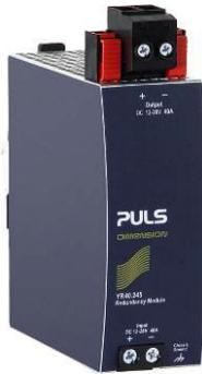
The YR40.245 is a 40 A single channel redundancy module, which is equipped with a plug connector on the output. The plug connector allows replacing the power supply or the redundancy module while the system is running. The plug connector prevents the output wires from touching and creating a short the load circuit.
