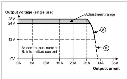
Fig. 6-2 Output voltage in "parallel use" mode, typ.
