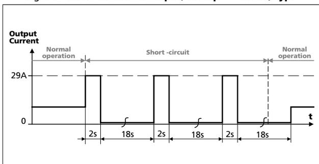
Fig. 6-4 Dynamic overcurrent capability, typ.
