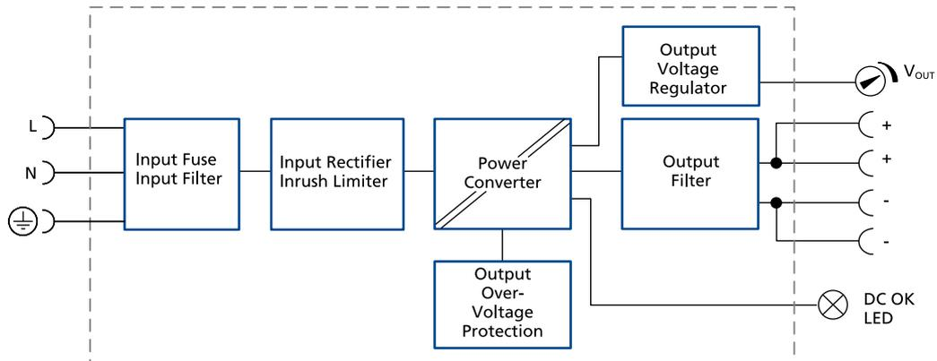
Fig. 11-1: Functional diagram
