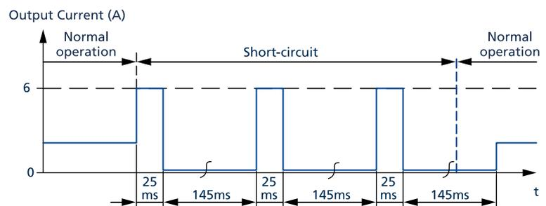
Fig. 6-2: Intermittent current at short circuit, typ.\*)
