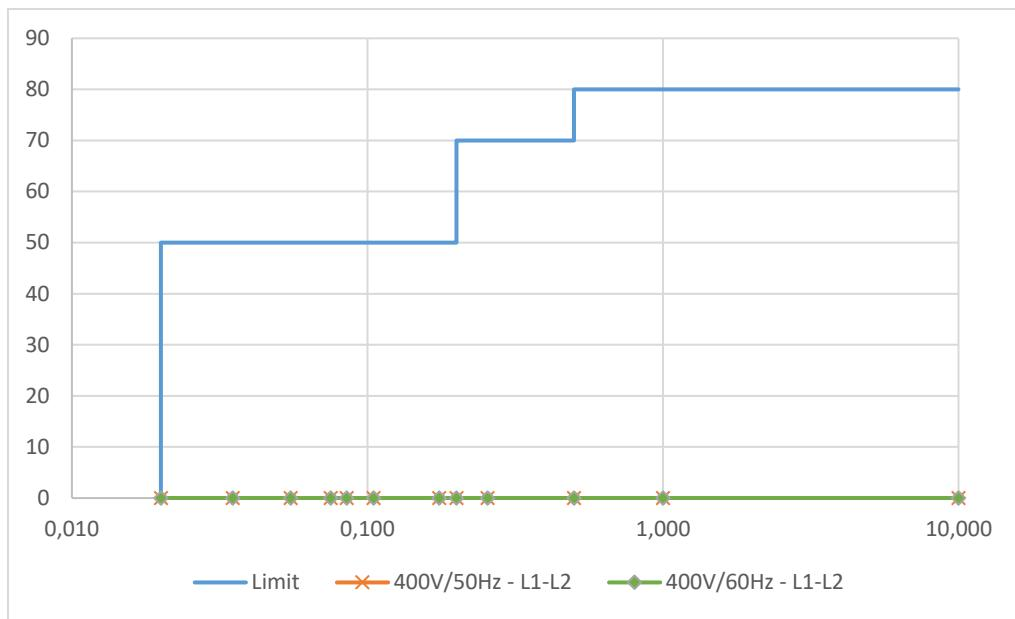
For all Sag times the voltage can be reduced to 0V without any influence on the output
